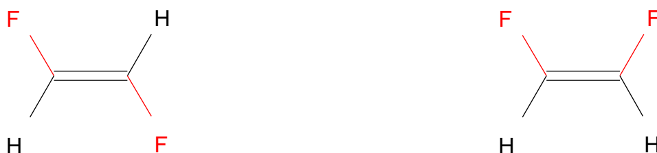
Figure 15: Structure of trans- and cis-difluoroethene, specified by the SMILES strings F/C=C/F (trans) and F/C=C\F (cis).
